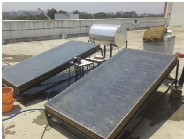
Fig. 4. Photo of comparison of smooth tube and dimpled tube concrete plate collectors
