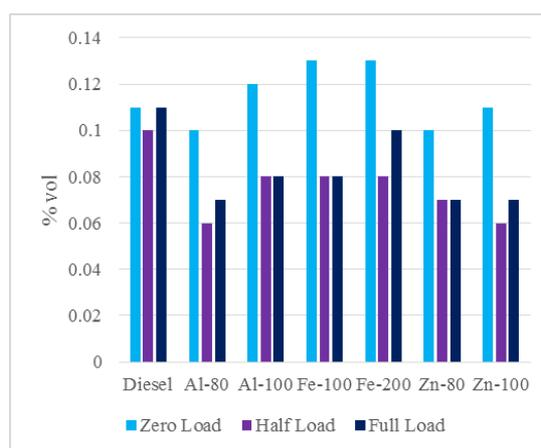
**Fig. 2** Variation of CO vs. loading at 180 bar
