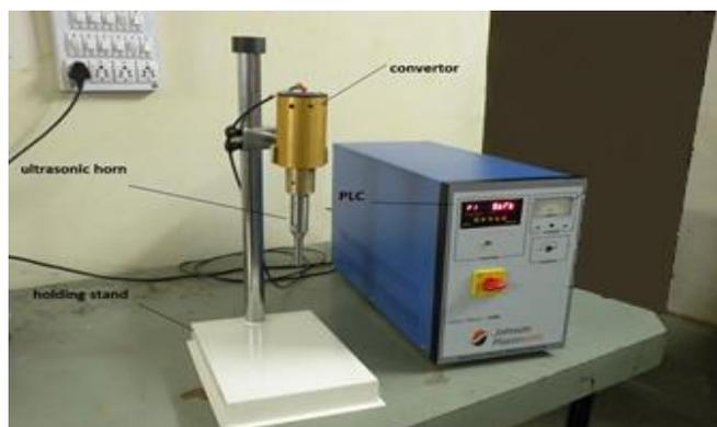
**Fig. 1** Probe Type Ultrasonicator
