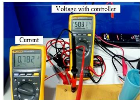
Fig. 11b. Experimental output values in rms with resistive loads ( R_1+R_2 )
