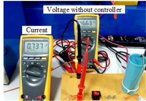
Fig. 11a. Experimental output values in rms with resistive loads ( R_1+R_2 )
