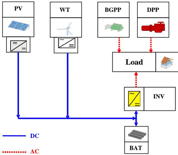
**Fig. 1.** Energy flows in the power supply system (PV – photovoltaic modules, WT – wind turbine, BGPP – biomass gasification power plant, DPP – diesel power plant, INV – inverter, BAT – battery).
