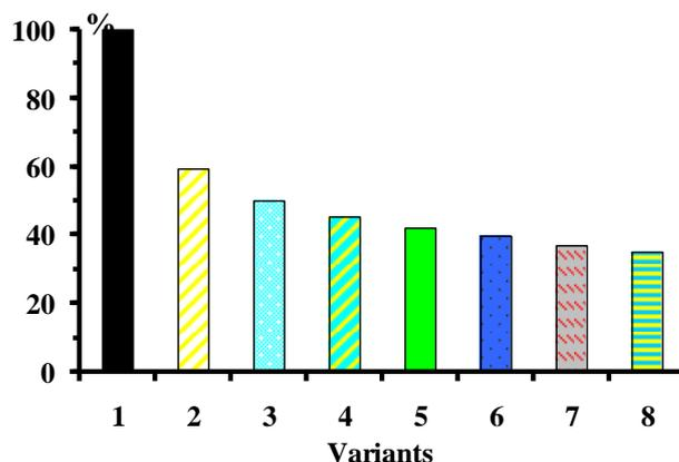
**Fig. 2.** Relative costs for different power supply system configurations (1 – DPP, 2 – DPP+PV, 3 – DPP+WT, 4 – DPP+WT+PV, 5 – DPP+BGPP, 6 – DPP+BGPP +PV, 7 – DPP+WT+BGPP, 8 – DPP+WT+PV+BGPP).
