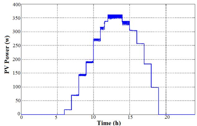
**Fig. 10 .** Output power of the PV panel
