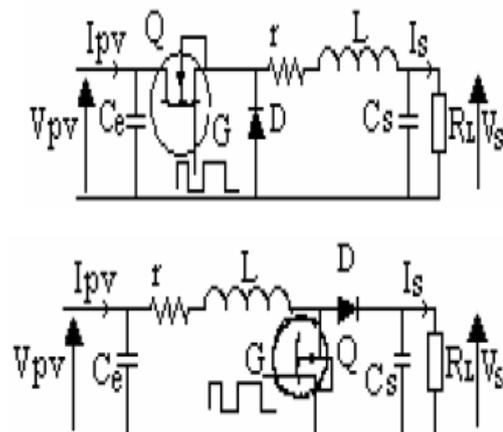
Fig. 3. DC/DC Buck and boost converter respectively used in photovoltaic system
