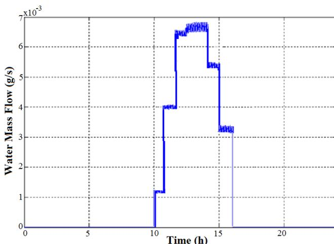
Fig.12. Mass flow of water injected into the PEM electrolysis
