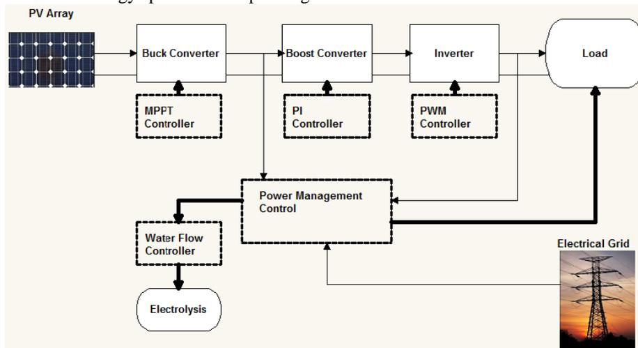
Fig.1. Schematic layout of the proposed PV/grid /electrolysis hybrid system with load
