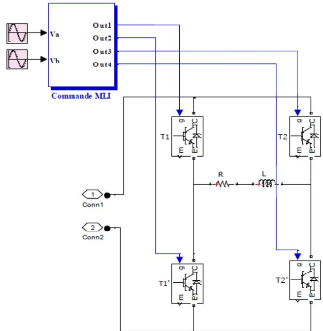
Fig. 5. Simulation diagram of the inverter and the RL load with the MLI command
