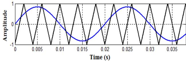
**Fig.7.** Sinusoidal MLI, generating control signals by a sinusoidal triangular carrier
