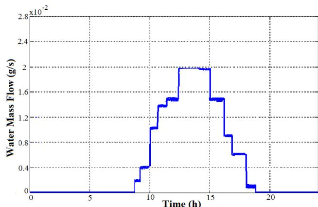
Fig.17. Mass flow of water injected into the PEM electrolysis
