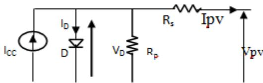
Fig. 2. Electrical design of the illuminated photovoltaic cell
