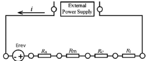
Fig. 4. The electrical circuit for the water electrolysis process
