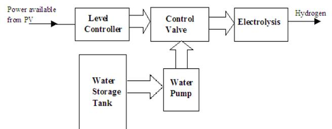
Fig. 6. Block diagram of water flow controller
