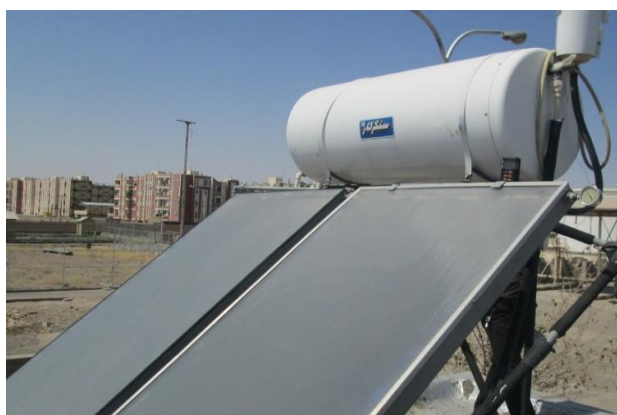
Fig. 4 Image of the FPC used in this study (image by Mohammad Javad Arabpour)
