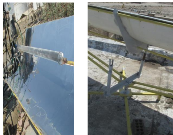
Fig. 3 The Manufactured PTC collector (image by Mohammad Javad Arabpour)
