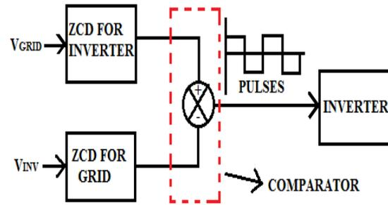
Figure 7. Generation of Pulses for Inverter from ZCD
