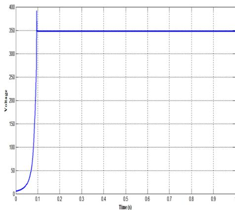
Figure 10. Output Voltage of Fly-back Converter
