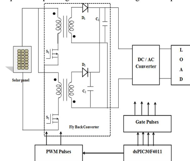
Figure 4.PV with Interleaved Converter
