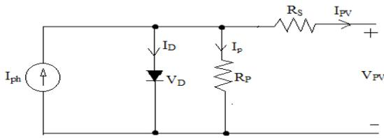
Figure 2. Single diode model of PV Cell
