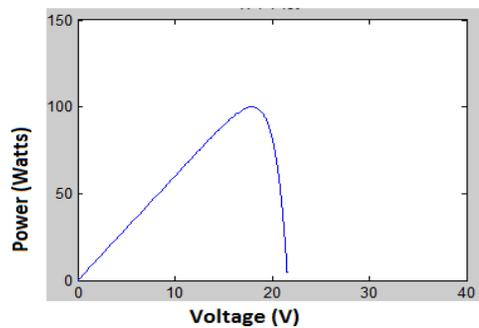
Fig2(b):P-V characteristics of PV system
