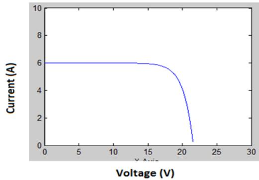
Fig 2(a):I-V characteristics of PV system
