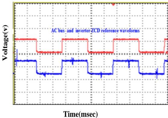
**Figure 13.** ZCD Outputs for Inverter and Grid (X-axis 1unit=5ms,Y-axis 1unit=5V)
