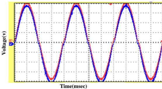
**Figure 14.** Grid synchronization waveform (In X-axis 1unit=5ms,Y-axis 1cm=60V)
