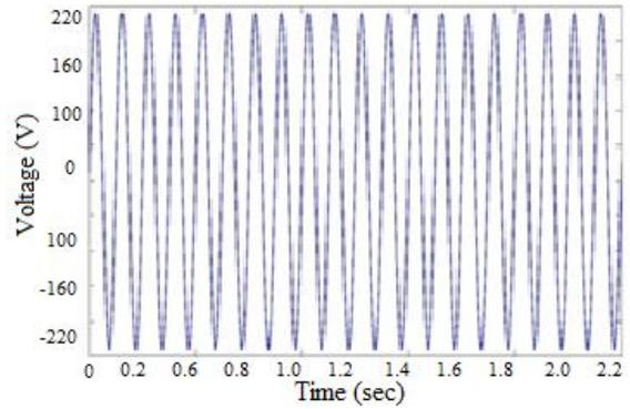
Figure 11. Inverter Output Voltage
