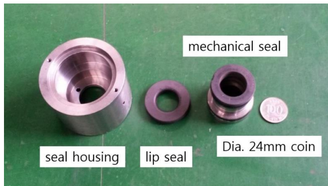
Fig. 7. Seal housing, mechanical seal and lip seal
