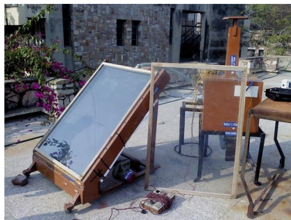
Fig.1. Photograph of solar air heater, cabinet dryer and two glazing frames
