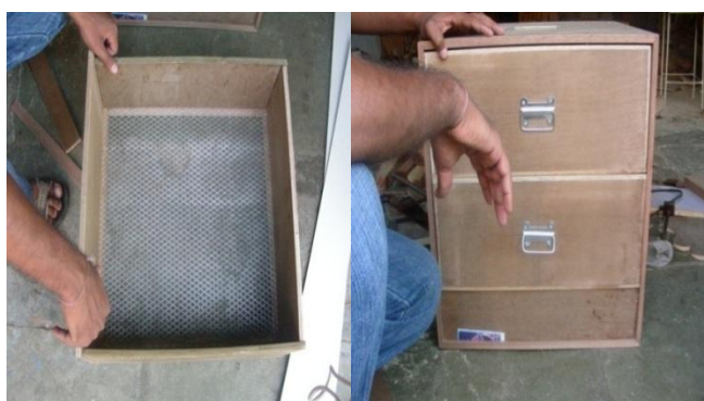
Fig. 2. Aluminum mesh used in shelf and two drawer shelves of drying chamber
