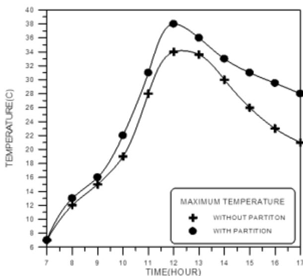
Fig.16. Influence of the barrier on the maximum temperature of the storage collector.
