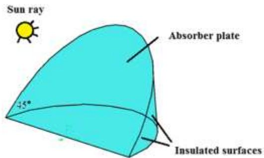
Fig. 4. Wedge storage collector.
