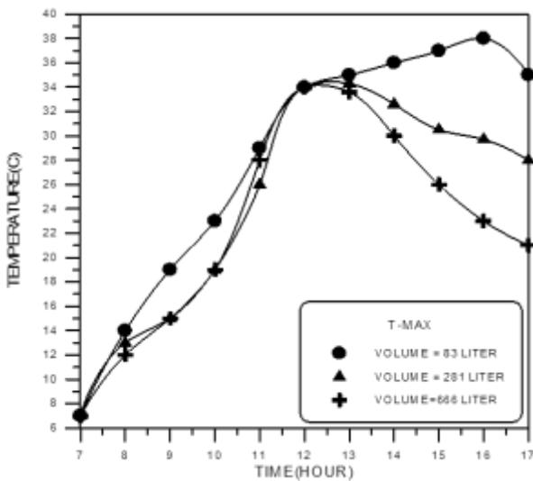
Fig. 9. Variation of maximum temperature of at the top of collector for different volumes.
