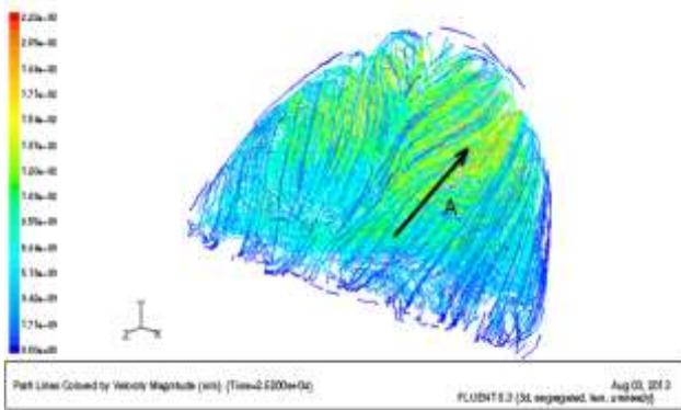
Fig. 12. Particle path lines in the front of the wedge collector
