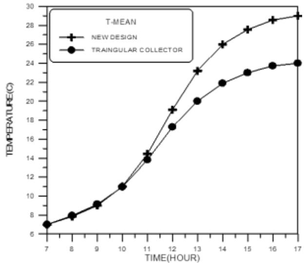
Fig. 10. Comparison of mean storage temperature for the wedge and triangular collectors (83 litres).
