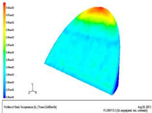
Fig. 17. Temperature distribution inside collector with the presence of a partition.
