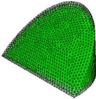
**Fig.4.** Mesh generated wedge collector by GAMBIT software.
