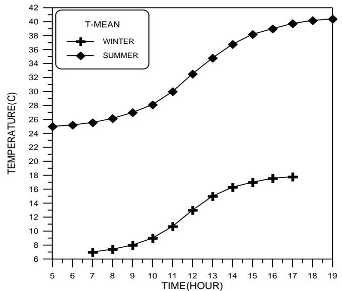
Fig. 7. Variation of mean storage temperature during a typical clear winter and summer.
