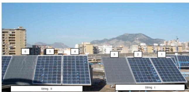
Fig. 5. Artificial shading on two modules of different strings [7].
