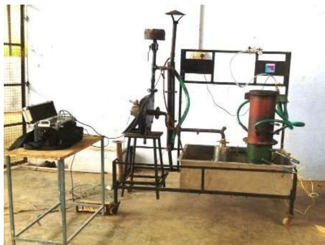
**Fig. 1:** Experimental setup for gasification and co-gasification studies
