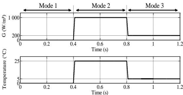
Fig. 8. Irradiance and temperature profiles of the PV generator
