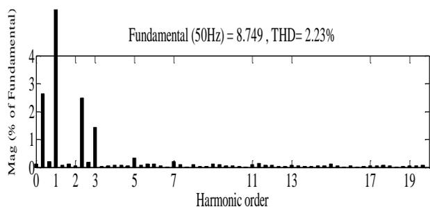
Fig. 22. Frequency representation of the current  $i_{ga}$  in Mode3
