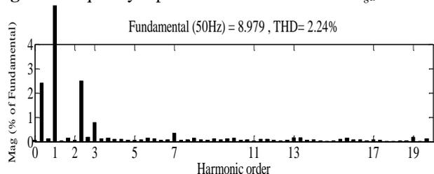
Fig. 23. Frequency representation of the current  $i_{gb}$  in Mode3
