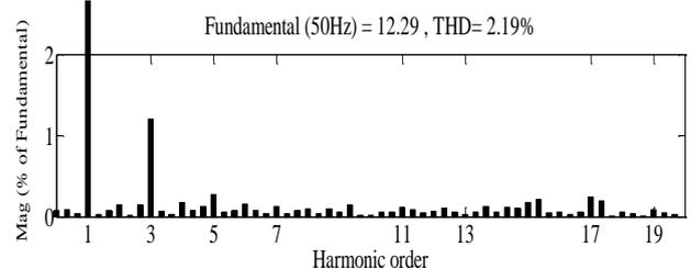
Fig. 19. Frequency representation of the current  $i_{gc}$  in Mode2
