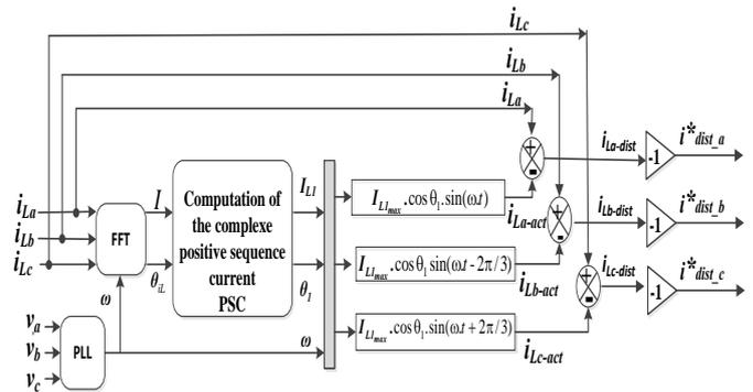
Fig. 4. Disturbing current generation block
