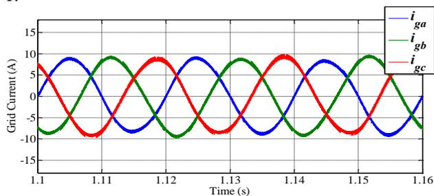
Fig. 21. Simulated three-phase grid current in Mode 3
