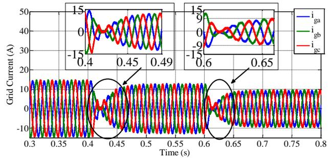
**Fig.30.** Dynamic response of the three-phase grid current with the proposed solar irradiation variation of Fig.32
