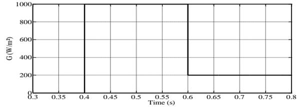
**Fig. 29.** Solar irradiance variation of the PV generator to study the dynamic response of the GCPVS
