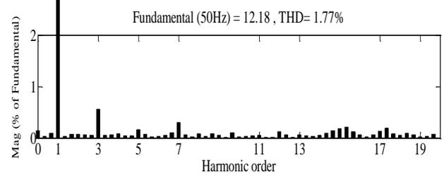
Fig. 18. Frequency representation of the current  $i_{gb}$  in Mode2
