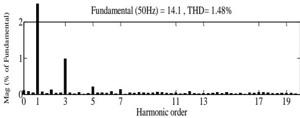
Fig. 12. Frequency representation of the current  $i_{ga}$  in Mode 1
