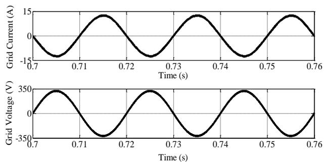
Fig.20. The Shape of the grid voltage and current of the phase "a" at the PCC in Mode 2
