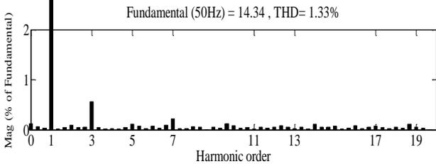
Fig. 13. Frequency representation of the current  $i_{gb}$  in Mode 1
