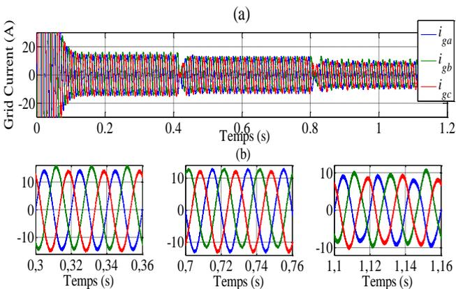
Fig. 34. Simulated three-phase grid current in the three operating modes in case of PQ theory(a) sample of 1.2 s (b) zoom on current wave in three modes
