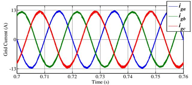
Fig. 16. Simulated three-phase grid current in Mode2
