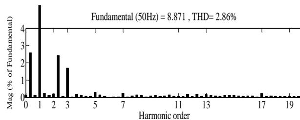
Fig. 24. Frequency representation of the current  $i_{gc}$  in Mode3
