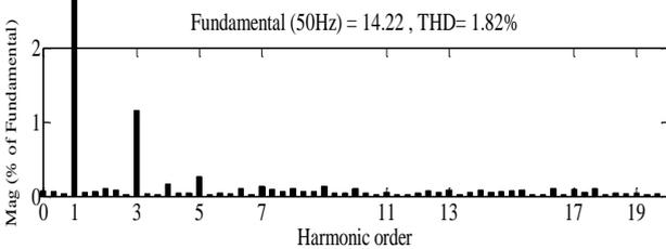
Fig. 14. Frequency representation of the current  $i_{gc}$  in Mode 1
