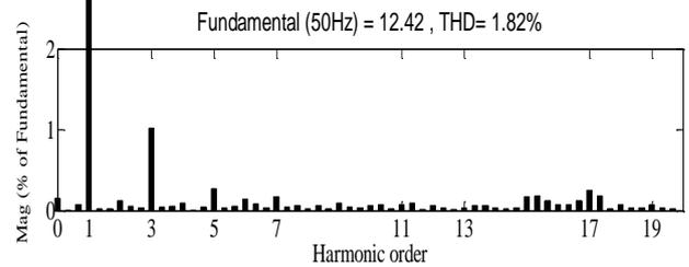
Fig. 17. Frequency representation of the current  $i_{ga}$  in Mode2
