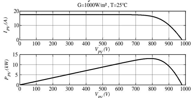
Fig. 2. Characteristics  $I_{PV} - V_{PV}$  and  $P_{PV} - V_{PV}$  of the used PV generator
