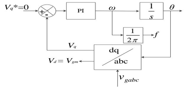
Fig. 5. Schematic diagram of the SRF-PLL
