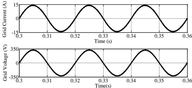
Fig. 15. The Shape of the grid voltage and current of phase "a" at the PCC in Mode 1
