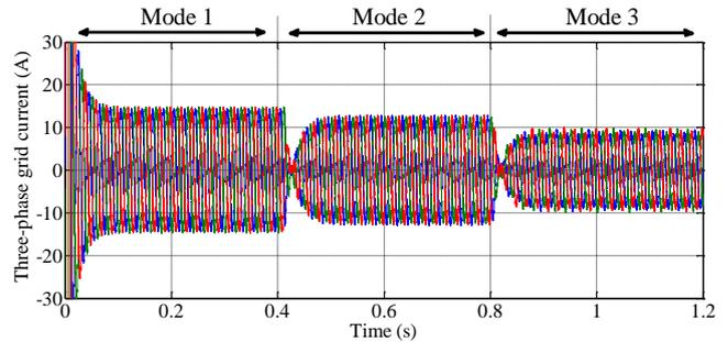
Fig. 10. Simulated three-phase grid current in the three operating modes
