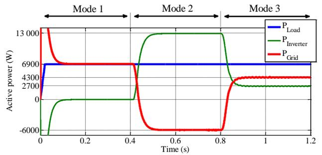
Fig. 9. Simulated active power of the load, PV inverter and the grid.
