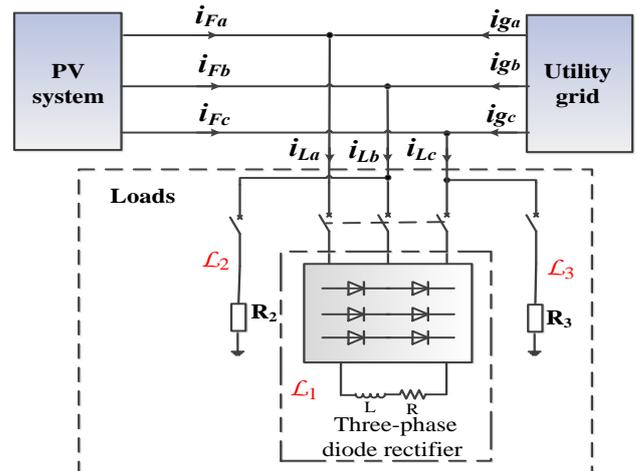
Fig. 6. Description of the three used loads connected at the PCC of the GCPVS
