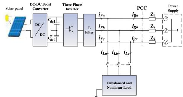
Fig. 1. The structure of the used grid tied photovoltaic system
