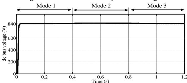
**Fig. 28.** The DC-bus voltage in the three operating modes
