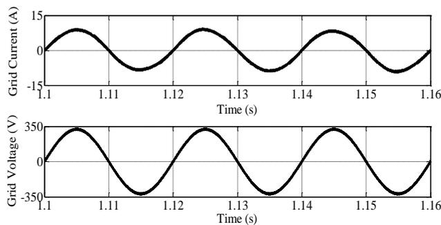
Fig. 25. The shape of the grid voltage and current of the phase “a” at the PCC in Mode 3
