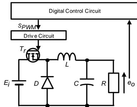
Fig. 7. Block diagram of digital control buck type dc-dc converter.
