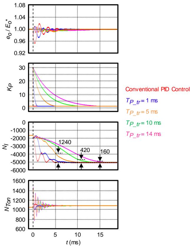
Fig. 11. Transient response of proposed method under changing  $T_{P\_tr}$ .
