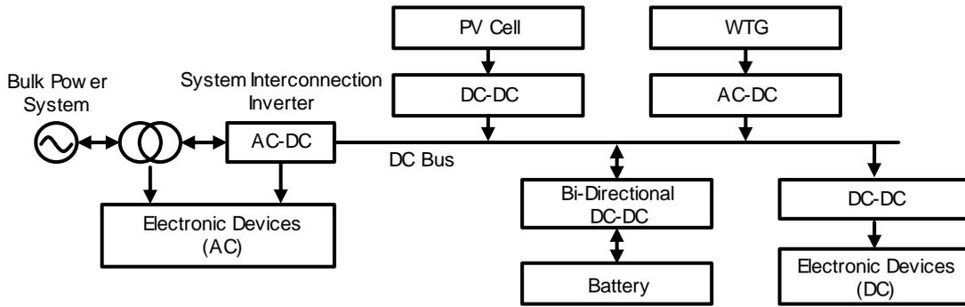
Fig. 1. General configuration of renewable energy system.
