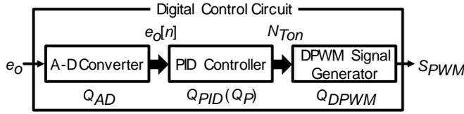
Fig. 2. General configuration of digital control circuit.
