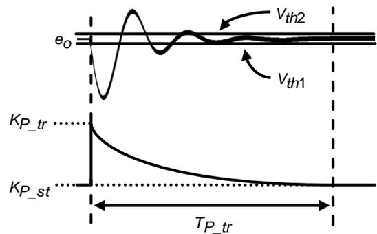
Fig. 9. Mechanism of the proportional gain changeable function.
