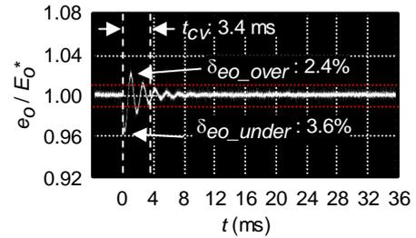
Fig. 5. Transient response of  $e_o$  ( $K_P = 1$ ,  $K_I = 0.01$ , and  $K_D = 1$ ).
