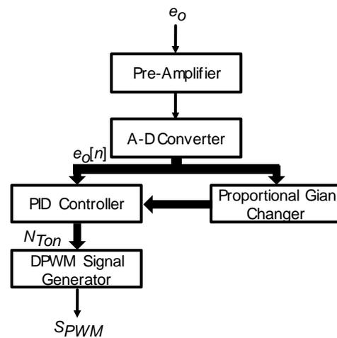
Fig. 8. Scheme of digital controller.
