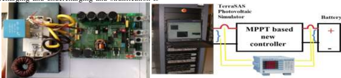
Fig. 7. (a) The developed charge controller, (b) Experimental set-up
