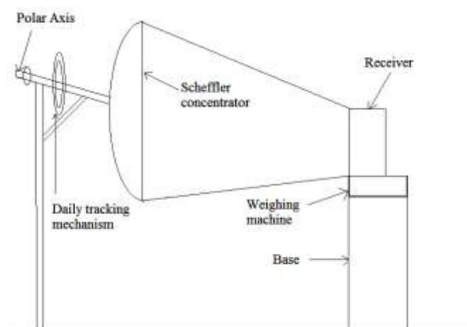
**Fig. 5.** Schematic diagram of the experimental setup
