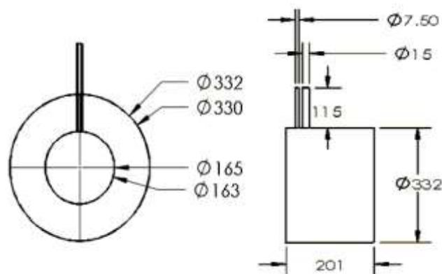
**Fig. 3.** Cylindrical receiver dimensions
