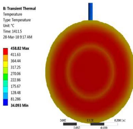
Fig 8(a). Temperature distribution on receiver without PCM while the dish is focused.
