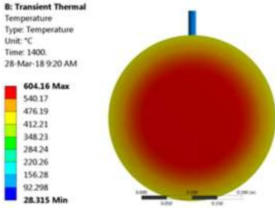
Fig. 8(b). Temperature distribution on receiver with PCM while the dish is focused.
