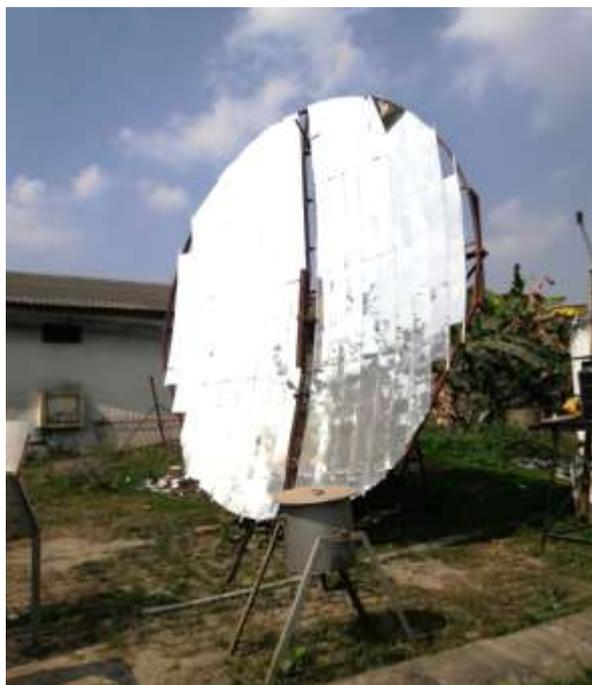
**Fig. 2.** Scheffler dish solar concentrator
