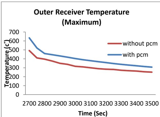
Fig 9(b). Maximum outer receiver Temperatures of the two receivers while the dish is defocused
