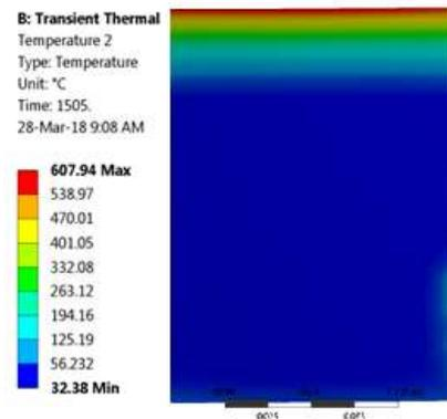
Fig. 10(b). Temperature distribution of water with PCM
