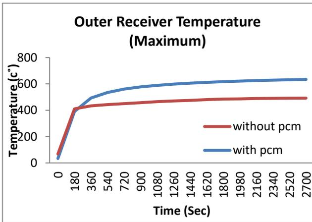
Fig 9(a). Maximum outer receiver Temperatures of the two receivers while the dish is focused
