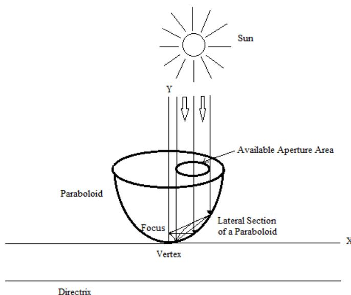
**Fig. 1.** Section of Scheffler reflector in a paraboloid
