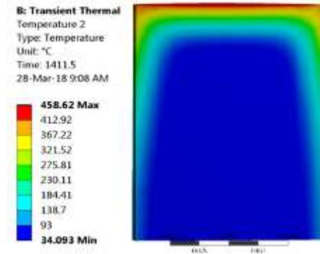
Fig. 10(a). Temperature distribution of water without PCM
