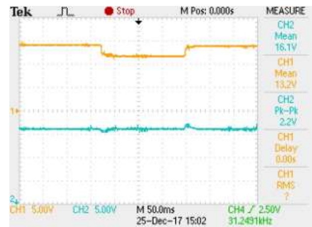
Fig. 17. Transient response with the load resistor (R) varying periodically stepwise between 50 and 100 Ω. CH1 (Top) battery voltage ( V_b ) (5 V/div). CH2 (Bottom) PV voltage ( V_p ) (5 V/div).
