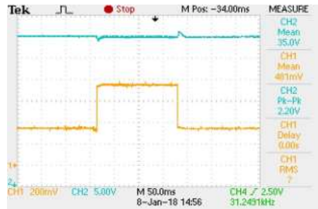
Fig. 14. Transient response with the load resistor (R) varying periodically stepwise between 50 and 100 \Omega . CH1 (Bottom) load current (200 mA/div). CH2 (Top) load voltage (5V/div). Load voltage tracks the desired 35-V reference well.
