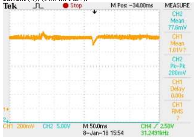
Fig. 16. Transient response with the load resistor (R) varying periodically stepwise between 50 and 100 Ω. CH1: Pv current ( x_1 ) (200 mA/div).
