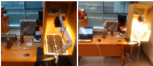
Fig. 11. Photo of the experimental platform of solar cells array electrical characterization system.
