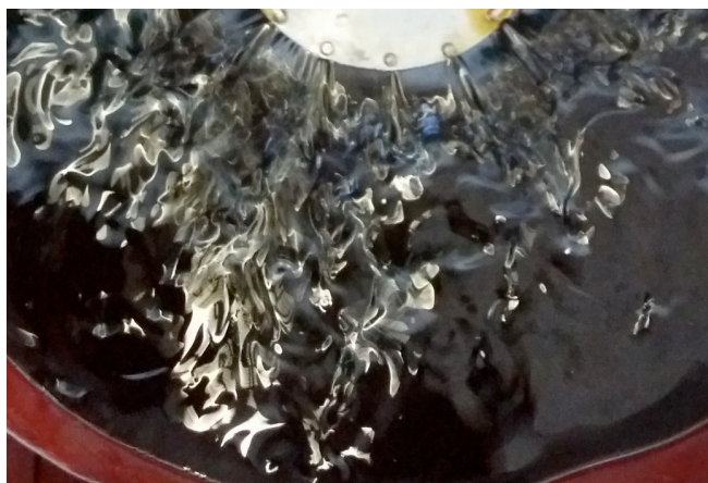
Fig. 8. The nature of the emulsion flow at a flow rate of 2.08 m/s, the clearance between the nozzle disks of 2 mm and a rotation speed of 1400 min -1
