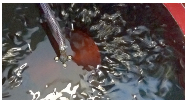
Fig. 10. The nature of the emulsion flow at a flow rate of 1.66 m/sec, the clearance between the nozzle disks of 2 mm and a rotation speed of 850 min -1
