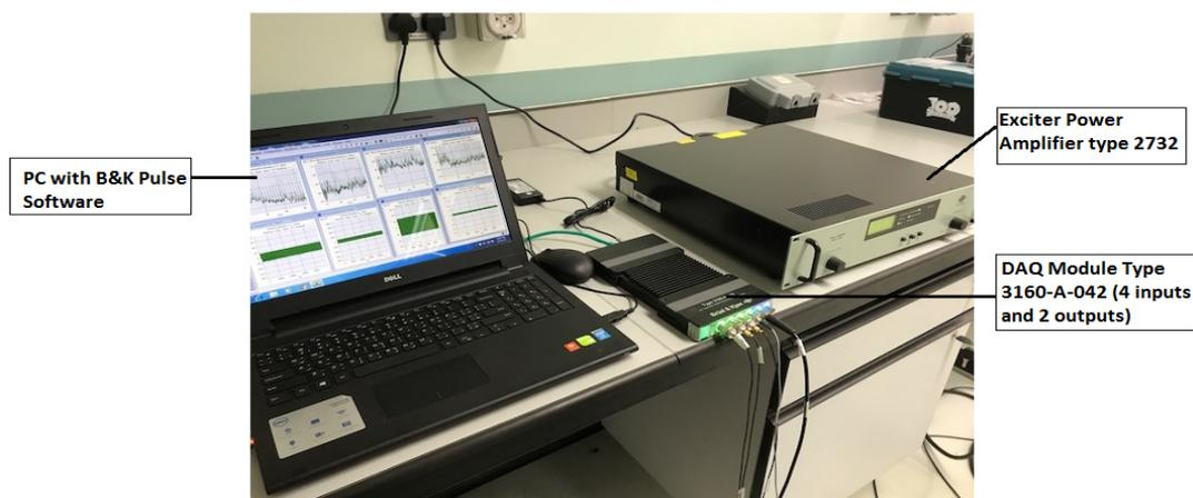
Fig.7. Shaker-Excitation experimental setup.
