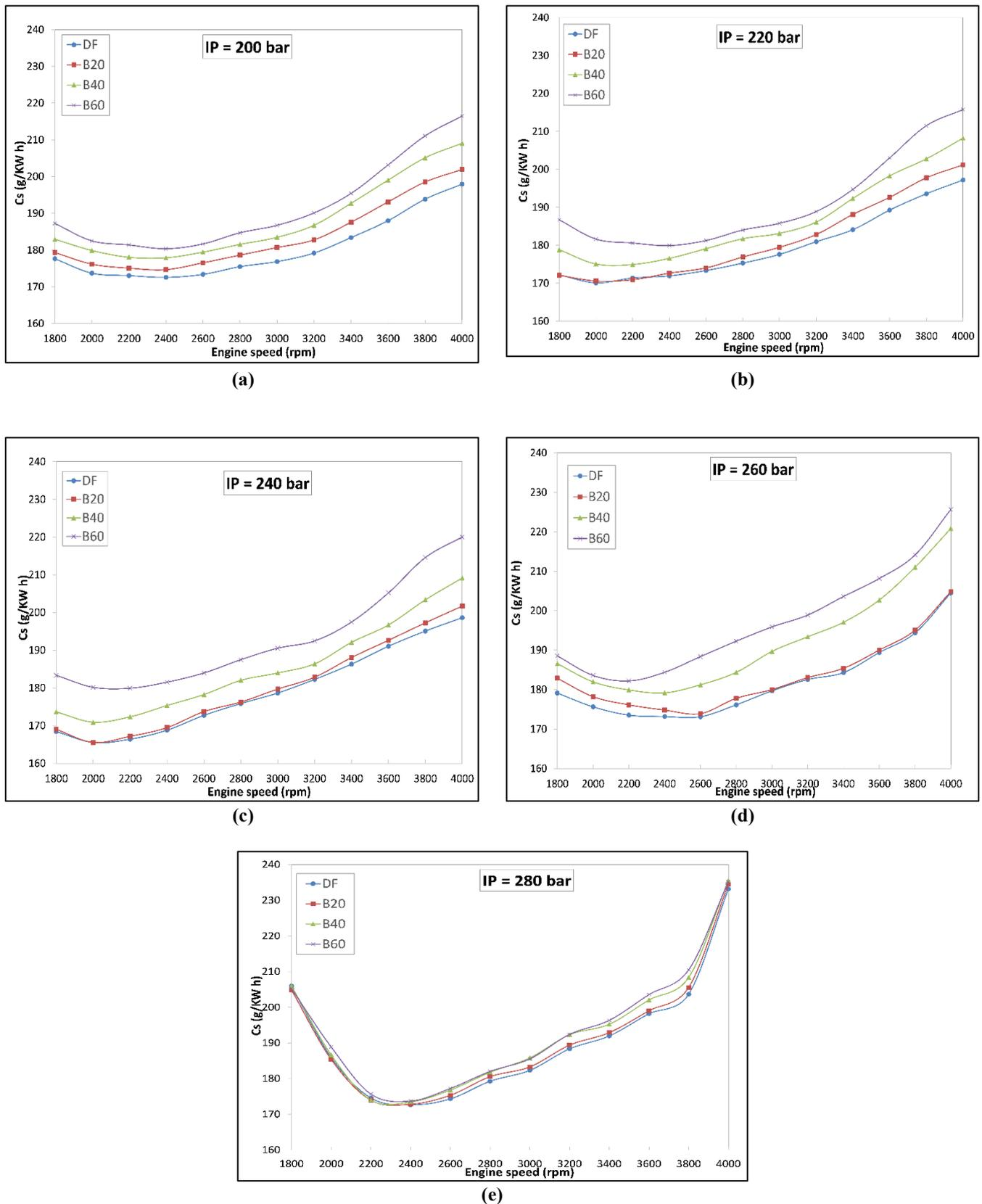
Fig.7. Specific consumption of DF and WCOME blends at different injection pressures
