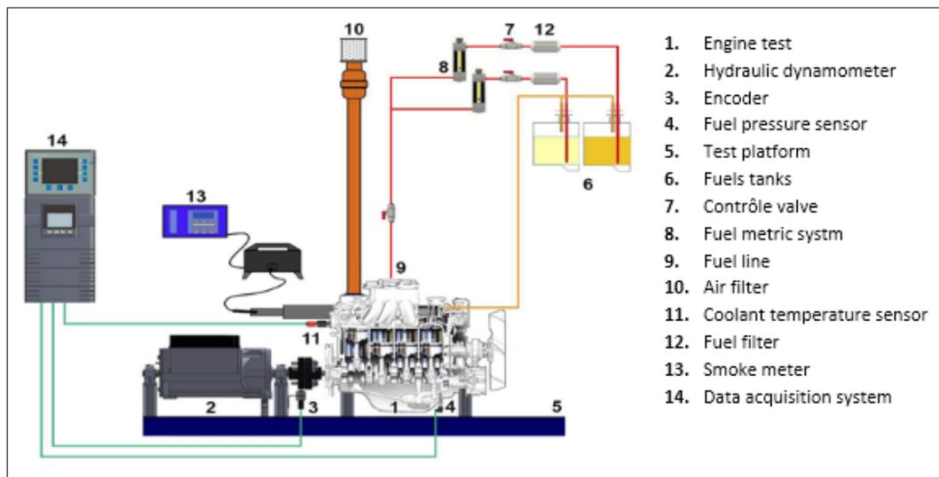
**Fig.3.** Schematic of experimental system
