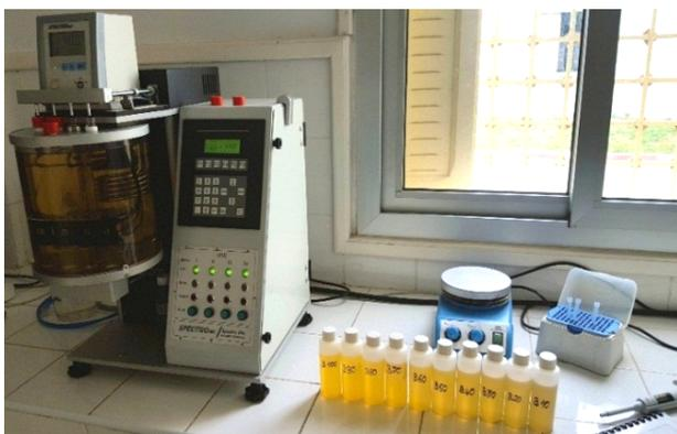
**Fig.1.** Kinematic viscosity measuring system
