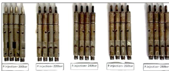
**Fig.4.** Sets of injectors used in tests
