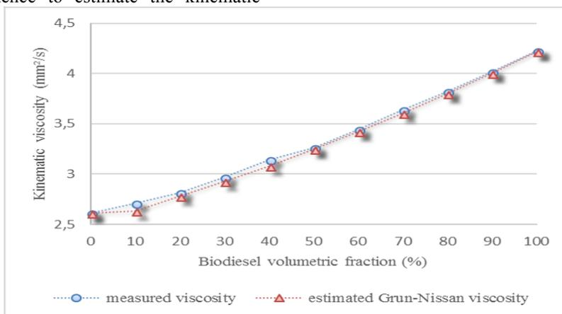
**Fig.2.** Kinematic viscosity variation with biodiesel fraction (measured and estimated)
