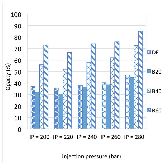
**Fig.8.** Variation of smoke emissions for different injection pressures
