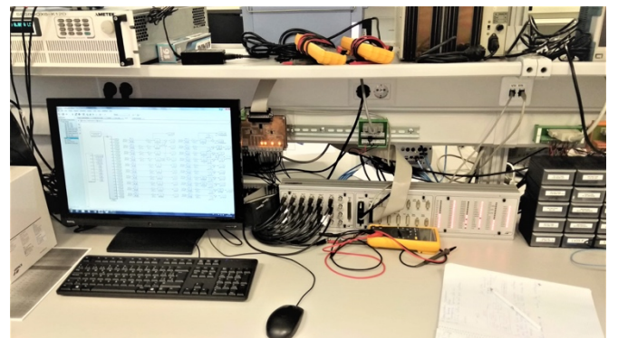
Fig. 5. AMREL SPS800X6-K12D DC source in the top-left and dSpace1103 real time platform in the centre.
