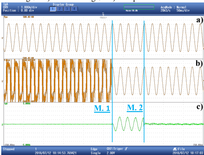
Fig. 7. First test chart: a) the voltage in the grid, b) the voltage in the three-phase system, c) the current injected into three-phase system from the HRES.
