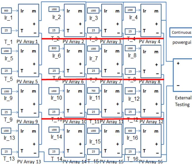
**Fig. 6.** Total cross tied (TCT) with bypass diode connection model
