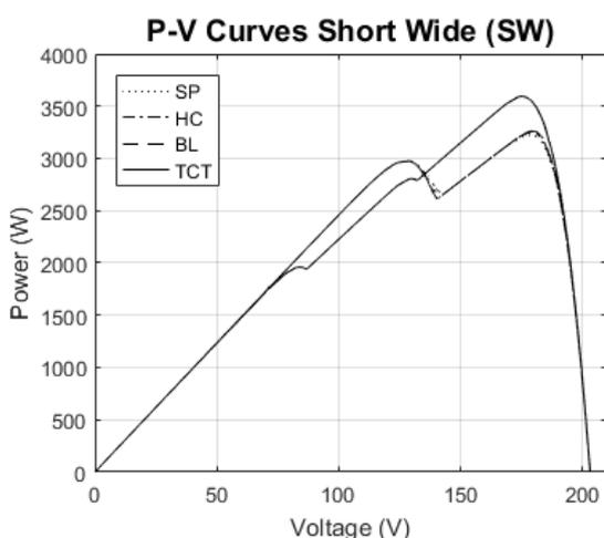
Fig. 9. P-V curves under short wide (SW) partial shading condition
