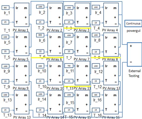
**Fig. 5.** 4x4 Bridge link (BL) with a bypass diode connection model
