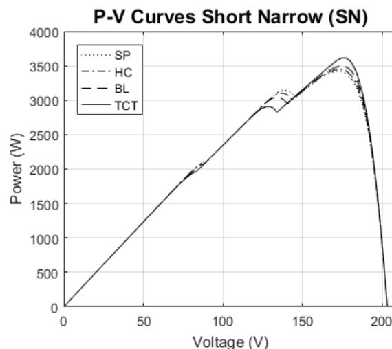
Fig. 10. P-V Curves under Short Narrow (SN) Partial Shading Condition
