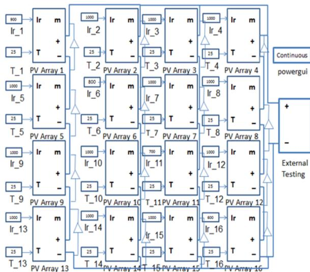
Fig. 3. 4x4 Series-parallel (SP) with a bypass diode connection model
