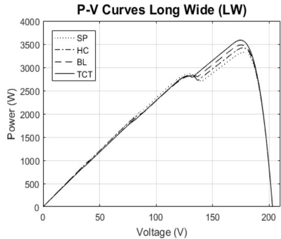
**Fig. 7.** P-V curves under long wide (LW) partial shading condition
