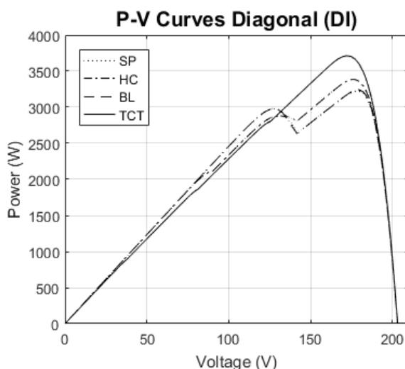
Fig. 11. P-V Curves under Diagonal (DI) Partial Shading Condition
