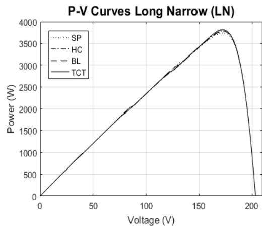
**Fig. 8.** P-V curves under long narrow (LN) partial shading condition
