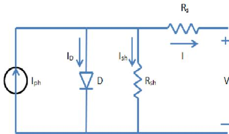
Fig. 1. Single diode equivalent photovoltaic cell model
