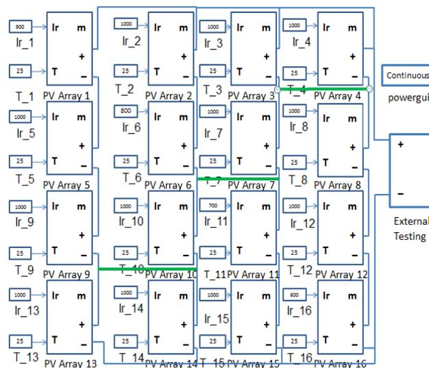
Fig. 4. 4x4 Honey comb (HC) with a bypass diode connection model
