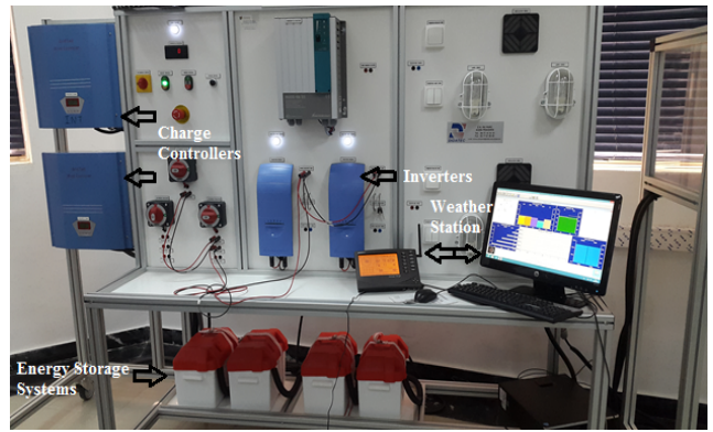
Fig.4. Microgrid site in Laboratory.
