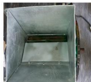
Fig. 7. Assembled novel cross-flow impulse turbine
