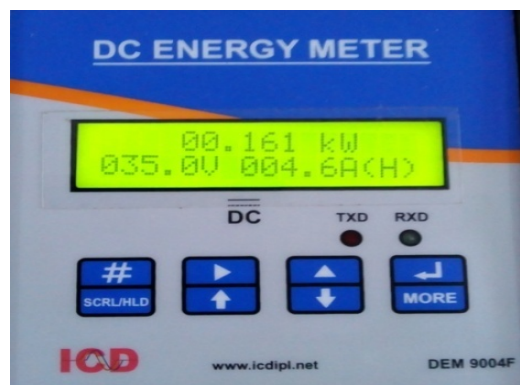
Fig. 14. Maximum power delivered by the emulated PV string
